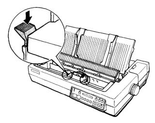
4. Turn the ribbon-tightening knob on the ribbon cartridge in the direction of the arrow.
